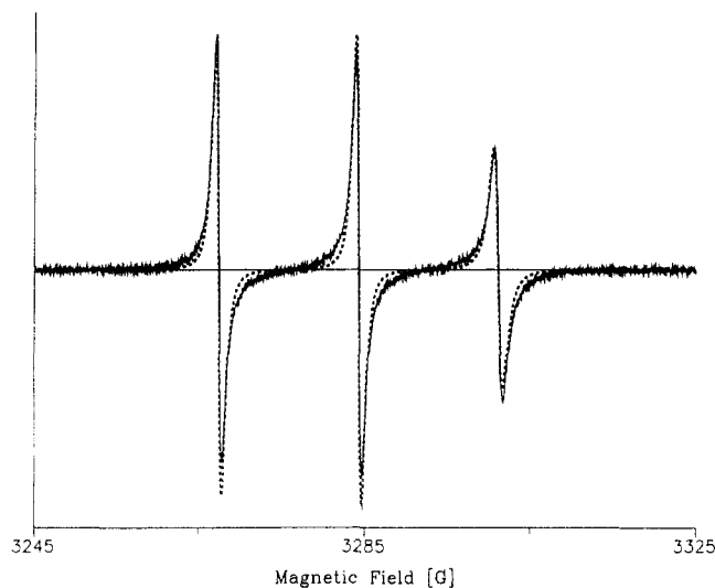
Figure 4. EPR spectrum of SL-PAA in dilute aqueous solution at \alpha = 0.0 measured at 353 K (—) and the simulated spectrum calculated using the parameters R_{\perp} = 1.3 and 10^8 \text{ s}^{-1} , R_{\parallel} = 4.8 \times 10^8 \text{ s}^{-1} , \vartheta = 40^\circ and \Delta H_{pp} = 0.06 \text{ mT} (---).
